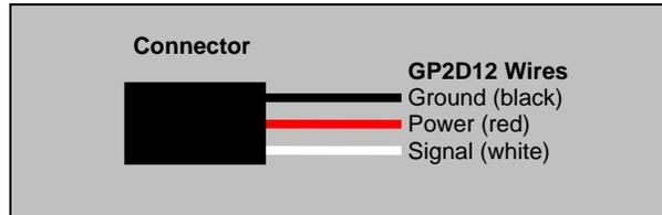
**Figure 6 - Range Sensor Connector**
