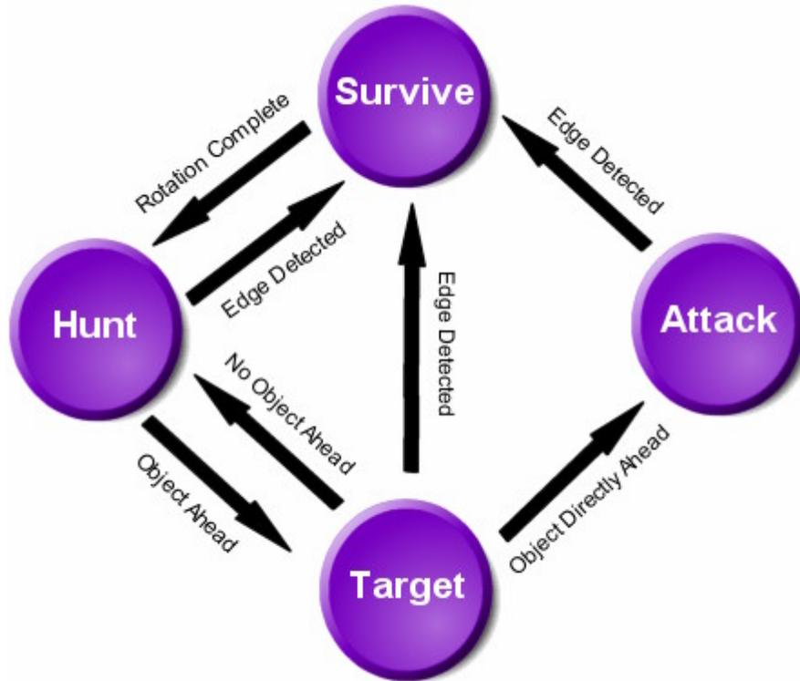
Figure 3 - Mini-Sumo Software State Machine
