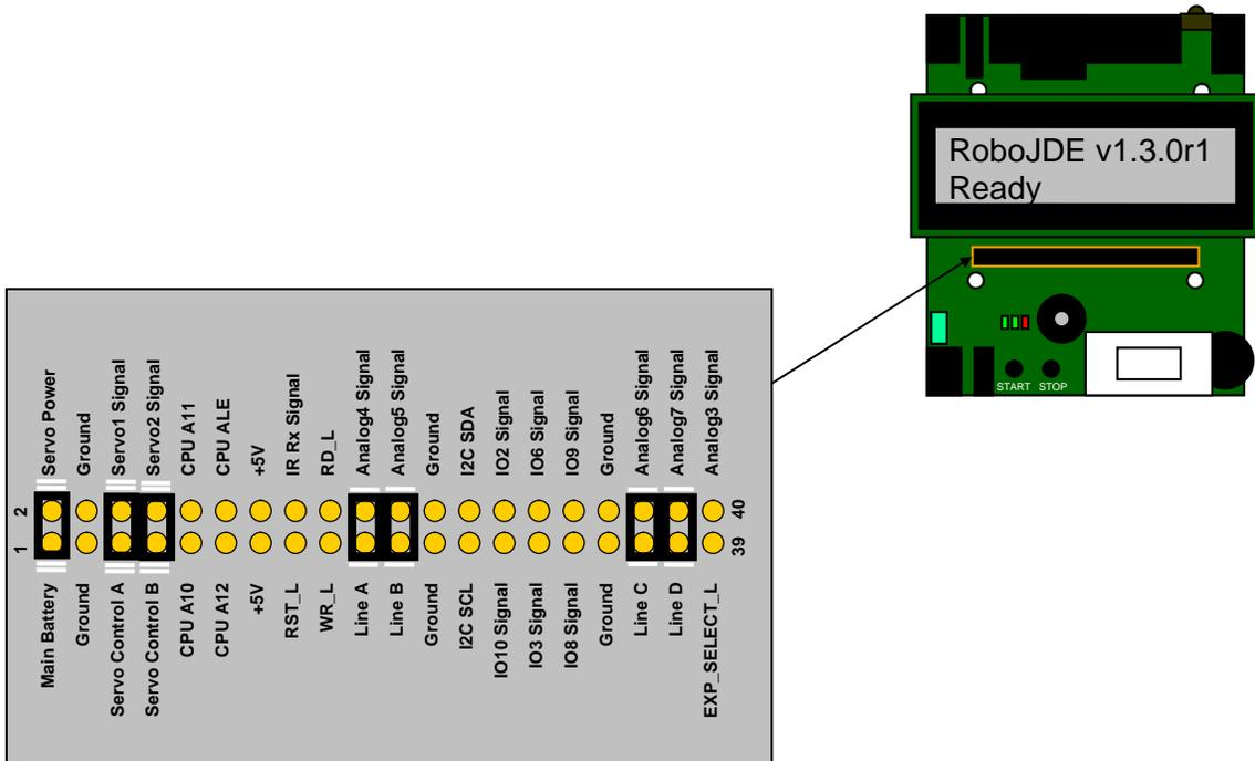
**Figure 7 - Expansion Header Jumpers**
