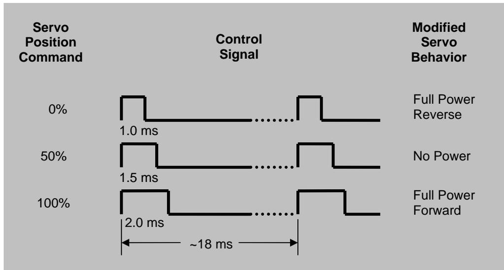
Figure 2 - Servo Control Signaling
