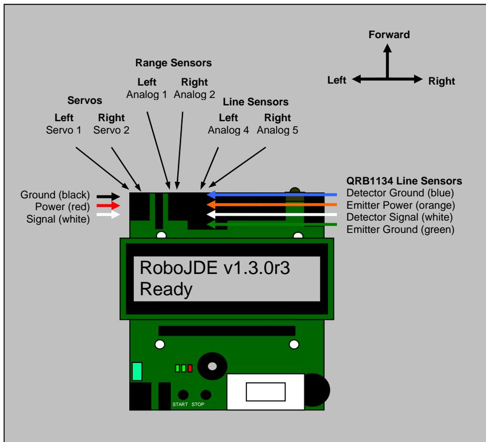
Figure 4 – Sensor and Servo Connections
